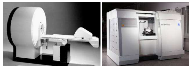
Figure 2. One of the first computed tomographs in medicine (left) and one of the first industrial computed tomographs (right)
