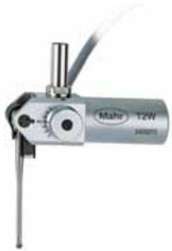
The inductive **T2W** probe is a universal device. The fact that the probe arm can be moved in a range of 180° and that there are a variety of clamping possibilities for the probe means that measurements can also be performed on difficult to access areas. You can combine easily exchangeable probe arms with a variety of styli in order to adapt the probe to the relevant measuring tasks or work-pieces.
