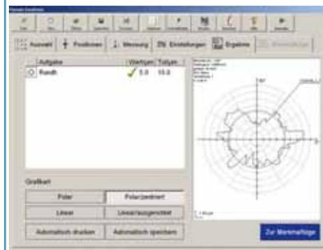
Workpiece alignment is supported by the computer. The measuring position is automatically recorded by the software. Detailed 3D graphics increase the informativeness of your measurement results. Moreover, you can also interactively rotate the graphic as desired for optimum presentation of the measurement result.
