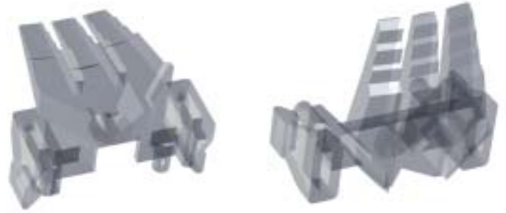
The light guide of a well-known automobile supplier – here the CAD data from the simulation software – was checked for proper operation using Metrotomography®.
